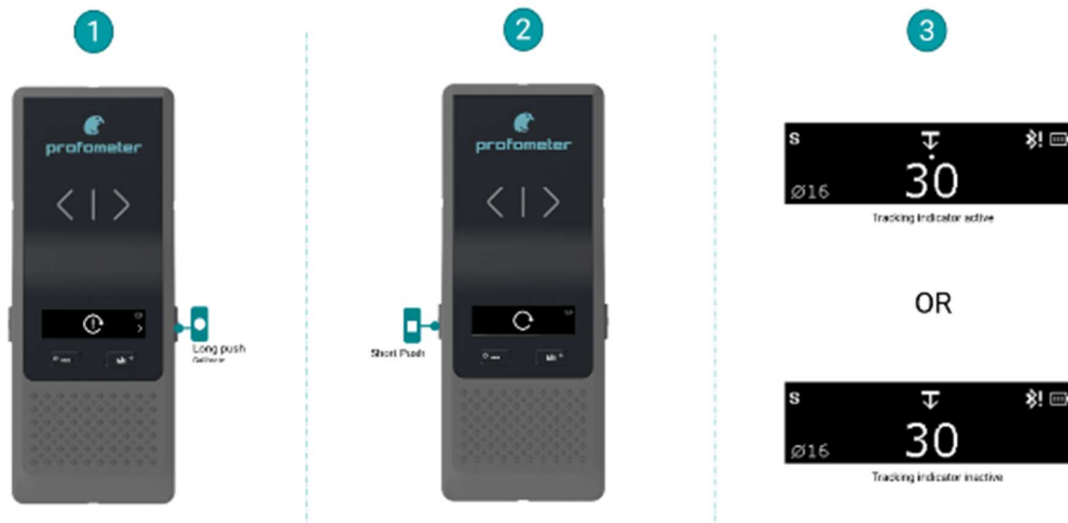
Figure 11: Activation or Deactivation of Tracking indicator
