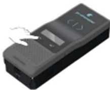
Figure 5 : Switching-on for standalone operation
