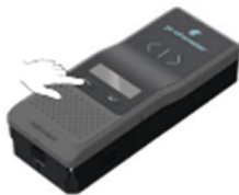
Figure 5 : Switching-on for standalone operation
