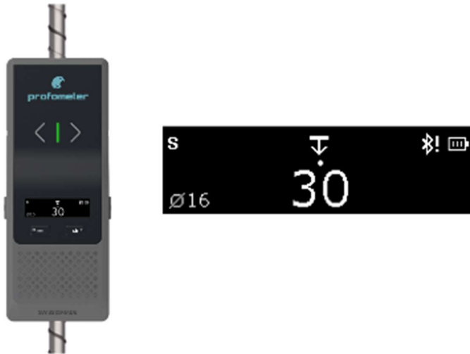
Figure 39: Indication of a rebar
