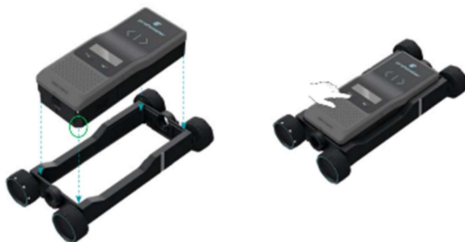
Figure 6 : Switching-on for connected operation
