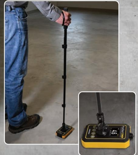
*Ergonomically measure without bending or kneeling with the optional Telescopic Extender*
