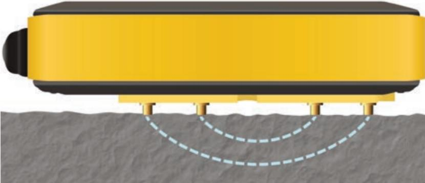
**NOTE:** It is suggested that the Meter operator take 3 - 4 measurements in close proximity to one another, noting the maximum measurement value for that inspection area. Using the **Hold Max** mode (pg. 3) makes this process rapid and convenient.
