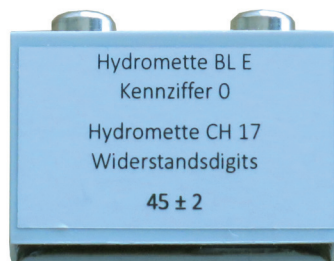
Examples for checking the Hydromettes CH 17 and BL E using the measuring cable MK 8 (order code 31006210)
